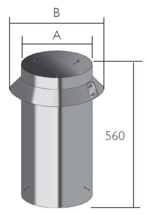
This component is used to protect the flue form accidental touch within the loft space, preventing a fire from starting.
