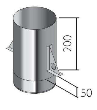
The lowering pipe is used to take the weight of up to  $15 \times 1$ m pipe lengths as they are lowered down the existing chimney stack.
