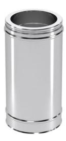
Pipes are available in various lengths. Each length is provided with a standard locking band. By adding a lip seal to the male end of the liner it can be used on positive pressure applications (P1). By adding a Pressure seal to the male end of the outer case, it can be converted for use on high positive pressure applications ICS5000)
