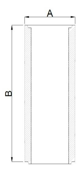
For lining masonry chimneys. Suitable for use in negative pressure (Dry Chimney) applications. CE Designation (T450 N2 D 3 G)
