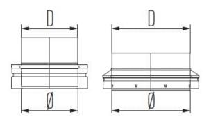
Reducing counter adaptor (D to be specified on order) - MFAC00 is part of our Starting components / adaptors, Twin Wall range for our Schiedel MF system, which is a modular twin wall insulated flue/chimney system, made of stainless steel, with a sealing ring.
