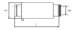
Resonance Silencer 30 dB (all welded) - MFSIR2 is part of our Silencers range for our Schiedel MF system, which is a modular twin wall insulated flue/chimney system, made of stainless steel, with a sealing ring.
