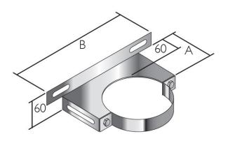
Retrofit Wall band - ICID Plus Support Components
