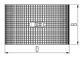
Spark arrester mesh - MEVV is part of the Schiedel ME range, which has a number of applications and advantages.
