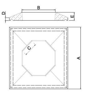
For DM Block Chimneys. Suitable for use in negative pressure (Dry Chimney) applications. CE Designation (T450 N1 D 3 G(00)
