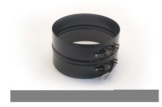
The Structural Locking Bands are purchased separately. It is used instead of a standard locking band in a situation where extra structural support is required. For example, where the chimney is 1.5m above the last support or above the roof. This also provides extra support in long horizontal runs. A max of 3m unsupported height can be achieved by fitting the structural locking band on the joint immediately below and on every joint above the last support.
