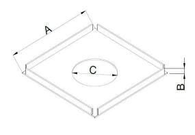
For supporting liners and support blocks when connecting to an appliance.
