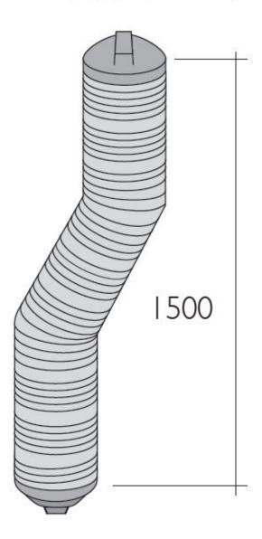
This kit is used as a test length prior to installing the main flex liner to ensure safe passage through the chimney for the liner. The video shows this Test kit in action.
