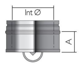
This item is used together with a tee on dry negative pressure applications to provide inspection or cleaning access.
