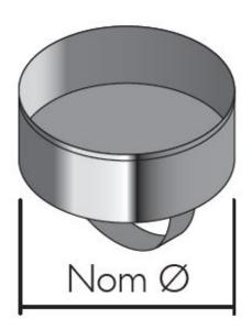
This item is used together with a tee on dry, negative pressure applications in order to provide inspection or cleaning access in a system.
