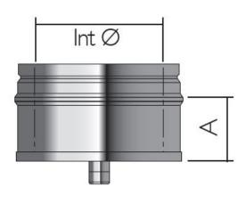
This item is used at the base of the vertical chimney to provide a drain off point for rainwater and condensate. It also provides inspection or cleaning access. It may be used in both dry and wet conditions and on both positive and negative pressure applications.
