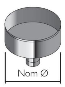
This item is used at the base of the vertical chimney to provide a drain off point for rainwater and condensate. It also provides inspection or cleaning access. It may be used in both dry and wet conditions and on both positive and negative pressure applications.
