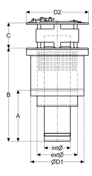
UK Plus Concentric flue system is a modular, high quality stainless steel concentric flue system for balanced flue applications.
