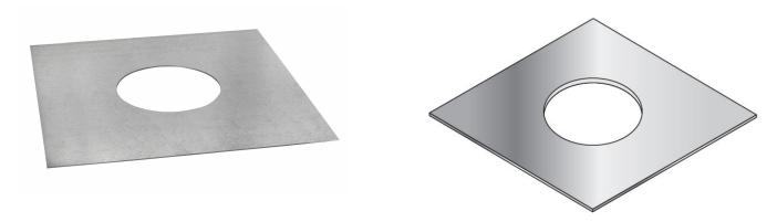
The top plate is used in combination with the top clamp to support the weight of the liner at the top of the stack. The top plate should be fixed securely in place and flaunched to make weather proof.
