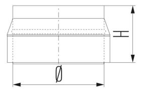
The Metaloterm UE system is a modular twin wall flue system, made of stainless steel with an air gap insulation and sealing ring.
