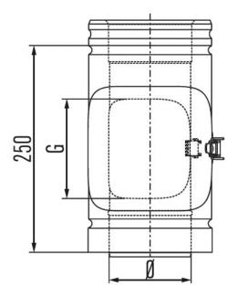
This component is part of the US flue system. US is a concentric system suitable for high temperature, non-condensing applications with flue gases in negative pressure.
