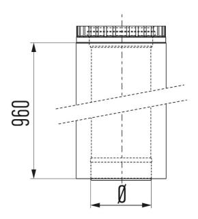
This component is part of the US flue system. US is a concentric system suitable for high temperature, non-condensing applications with flue gases in negative pressure.
