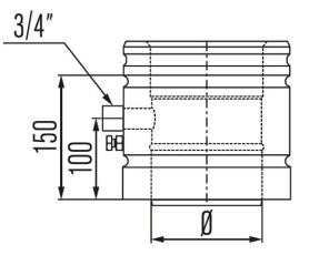
This component is part of the US flue system. US is a concentric system suitable for high temperature, non-condensing applications with flue gases in negative pressure.
