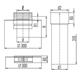
This component is part of the US flue system. US is a concentric system suitable for high temperature, non-condensing applications with flue gases in negative pressure.
