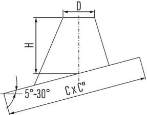
This component is part of the US flue system. US is a concentric system suitable for high temperature, non-condensing applications with flue gases in negative pressure.
