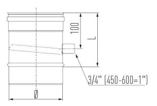
Condensate collector with drain - MEEMC is part of the Schiedel ME range, which has a number of applications and advantages.
