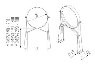
Wall band adjustable 90 - 200 - MEMBV2 is part of the Schiedel ME range, which has a number of applications and advantages.
