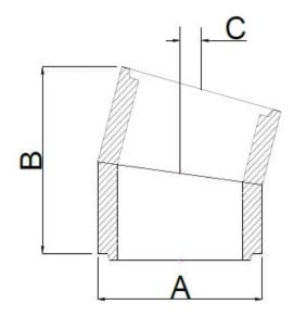
For lining masonry chimneys. Suitable for use in negative pressure (Dry Chimney) applications. CE Designation (T450 N2 D 3 G)
