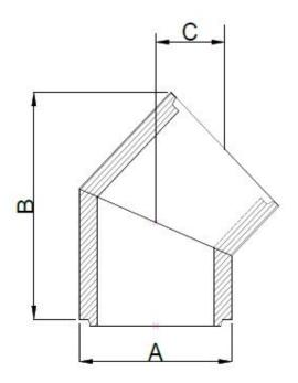
For lining masonry chimneys. Suitable for use in negative pressure (Dry Chimney) applications. CE Designation (T450 N2 D 3 G)
