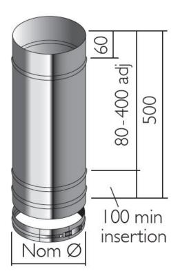
This item provides for an adjustable pipe length in the Prima Plus range. It is provided with a cover band to cover the joint in the middle of the pipe. Suitable for use without any gaskets in negative pressure (N1) applications.
