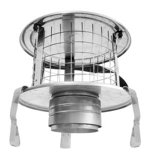
This updated design of the Pot hanger in the key  $\emptyset$ 125 and  $\emptyset$ 155 diameters brings additional strength with mesh included as standard; one piece looped straps fasted with bolts to the terminal cap and spot welded to the mesh, and Schiedel's tested and approved screwfit design ensuring that this pot hanger and terminal can bear the weight of up to 15m of TecnoFlex Plus liner.
