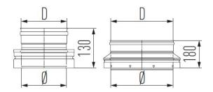
Counter adaptor - MFAC is part of our Starting components / adaptors, Twin Wall range for our Schiedel MF system, which is a modular twin wall insulated flue/chimney system, made of stainless steel, with a sealing ring.
