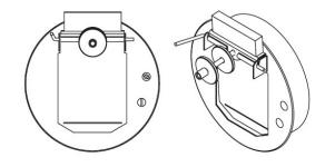
Draught stabiliser, adjustment range from 10 till 25 Pa - MENLT is part of the Schiedel ME range, which has a number of applications and advantages.
