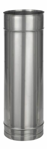
Available in lengths from 1000mm – 200mm. Suitable for use without any gaskets in negative pressure (N1) applications. By adding a lip seal gasket to the male end of the liner it can be used on positive pressure applications (P1).
