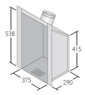
This item is a single wall design with sloping back to help fit some openings. For radiant gas fires complying with BS7977-1.
