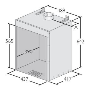
For use with Inset Live Fuel Effect gas fires complying with BS 7977-1, with a heat output not exceeding 7kw.
