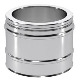
Pipes are available in various lengths. Each length is provided with a standard locking band. By adding a lip seal to the male end of the liner it can be used on positive pressure applications (P1). By adding a Pressure seal to the male end of the outer case, it can be converted for use on high positive pressure applications ICS5000)
