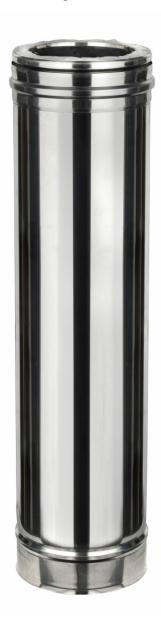
Pipe 750 Effective Length - ICS Pipes. ICS is converted into ICS Plus by adding a lip seal to each component with a male form on the liner. This creates a twin wall insulated chimney system designed for the new generation of condensing gas and oil appliances, with continuous operating temperatures up to 200°C, short firing up to 250°C, and positive pressure up to 200pa at the appliance outlet.
