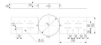
The Metaloterm UE system is a modular twin wall flue system, made of stainless steel with an air gap insulation and sealing ring.
