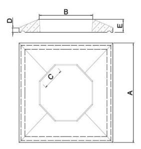
For DM Block Chimneys. Suitable for use in negative pressure (Dry Chimney) applications. CE Designation (T450 N1 D 3 G(00)
