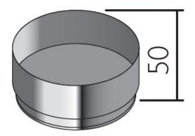
This item is used together with a tee on dry, negative pressure applications in order to provide inspection or cleaning access in a system.
