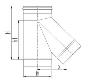
Tee-piece 45 Degree with condensate deflector - MET 45 is part of the Schiedel ME range, which has a number of applications and advantages.
