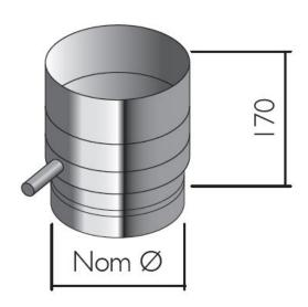
This article allows may be used in the vertical or in a horizontal run. It catches condensate as it runs down the chimney system and allows it to be safely drained off without running back into the appliance.
