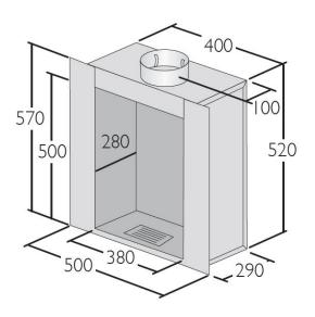
This item has a twin wall construction for reduced condensation. Otherwise as VRV Single Skin Box.
