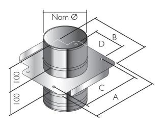
This item is used to support a wall mounted system. It is used in combination with either side plates or cantilever brackets (see below). Suitable for use without any gaskets in negative pressure (N1) applications. By adding a lip seal gasket (See S000 and V000 at the bottom of this page) to the male end of the liner it can be used on positive pressure applications (P1).
