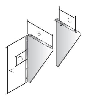
The Side plates are used in combination with a Wall Support Top Plate at the base of a wall mounted system or as an Intermediate Wall Support. They may be installed with the points upwards (in traction) giving the best load bearing capacity or with points downwards (See Load bearing Section)
