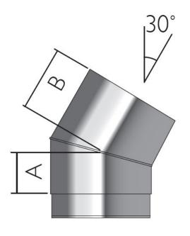
This item gives a fixed angle of 30 deg and when used in pairs gives a 30 deg offset in the connecting  $\rightarrow$  flue pipe. Suitable for use in negative pressure (N1) applications.
