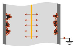
4. The fine dust collects on the inner wall of the chimney.
