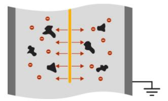
2. Electrons are released by means of a high voltage electrode.
