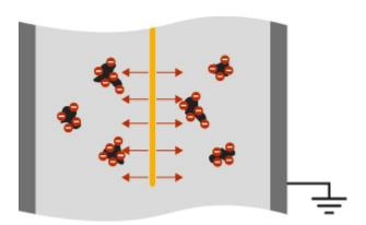
3. The electrostatically charged particles move to the chimney's inner wall.
