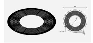
The ventilated firestop plate is used where Permeter Smooth Air will be running through a bedroom or other living space where the chimney will be enclosed in a shaft.
