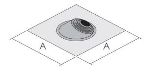
This item is manufactured with a malleable base and a EPDM or Silicon cone is used to provide a water tight flashing around the chimney as it passes through a roof pitched between 0-45 degrees. The cone is subdivided by diameter and a range of diameters is covered by each of the three flashings available in the range. The cone is cut down to the predetermined diameter size to fit the outer case of the chimney.
