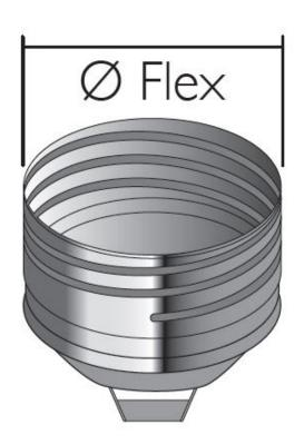
This component screws onto the flexible liner and rope ties to the nose loop. The flex can then be pulled down the chimney.
